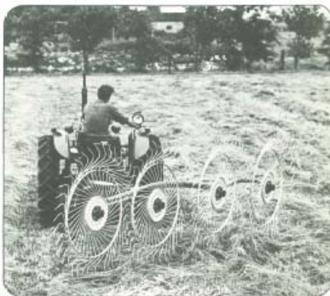
The floating fingerwheels with their flexible lines gently collect all the crop from the stubble as well as the hollows.
